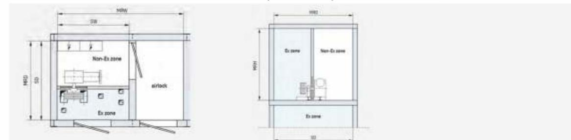
MACHINE ROOM WITH EXPLOSION PROTECTION (FULL Ex), ATEX
