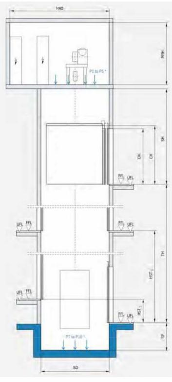
\*THE EXACT POSITIONS OF THE LOAD POINTS IN THE MACHINE ROOM AND IN THE SHAFT PIT ARE ENTERED IN THE GENERAL ARRANGEMENT DRAWING.
